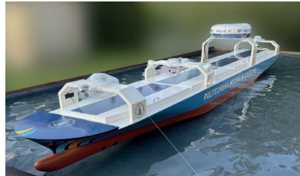
Scale model of the Triple E container ship „MAJESTIC MAERSK”, 18,340 TEU - scale 1:70
